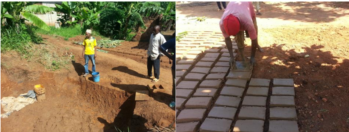
Figure 3: Production process of mud bricks
