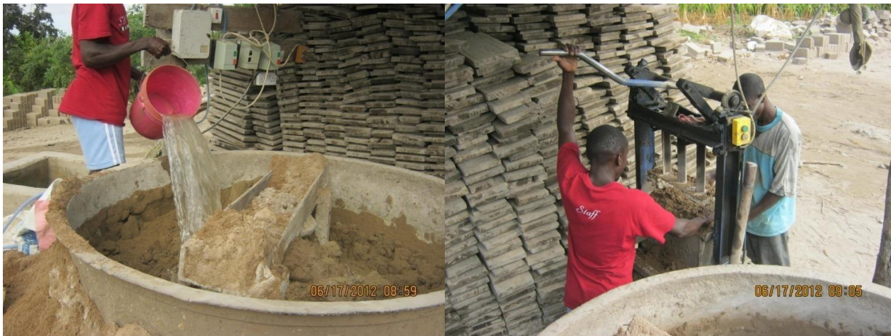
Figure 5: Production of sand cement blocks
