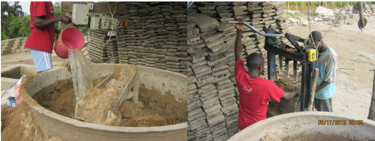
**Figure 5: Production of sand cement blocks**
