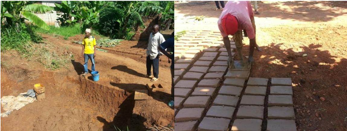
**Figure 3: Production process of mud bricks**
